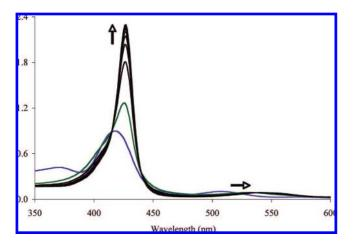
*Figure 5.* Reaction of [Fe(TPP)Cl] with 2 in THF without illumination. The Soret band for [Fe(TPP)Cl] (purple trace) shifts hypsochromically and increases in intensity upon addition of 2 (green trace). Scans every 60 s thereafter (black traces) show increasing absorptivity that is complete within 10 min.
