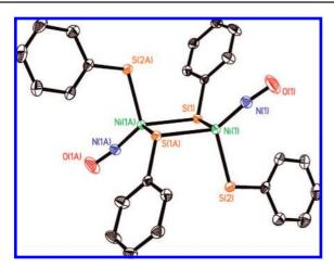
*Figure 2.* ORTEP diagram showing 50% probability thermal ellipsoids and selected atom labels for **3**. The  $Et_4N^+$  cations, H atoms, and disordered CH<sub>3</sub>CN have been omitted for clarity. Selected bond distances (Å) and angles (deg): N1–O1, 1.168(3); Ni1–N1, 1.657(2); Ni1–S1, 2.2923(9); Ni1–S1A, 2.3320(10); Ni1–S2, 2.2733(11); Ni1–N1–O1, 161.5(2); S1–Ni1–N1, 118.56(8); S1A–Ni1–N1, 127.12(9); S2–Ni1–N1, 116.58(8); S1–Ni1–S1A, 89.24(4); S1–Ni1–S2, 100.80(3); S1A–Ni1–S2, 98.65(3).
